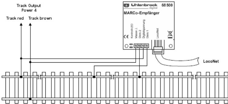
**NOTE:** If multiple boosters are used take care to ensure that the chassis side of the supply transformers are coupled so as to perform without interference.
