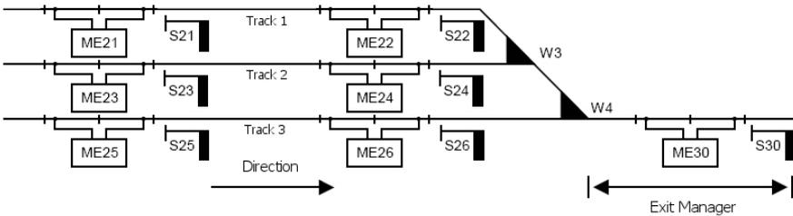
In the example, the Exit Manager needs to selectively switch the signals associated with each of the block sections in the station. It is no longer sufficient, like in the previous example, to switch route when the train at the Exit Manager to switch all signals in the station to “red”, e.g. a train from track 1 reaches the Exit Manager, then signal 22 must be switched to “red” and signal 21 to “green”.
