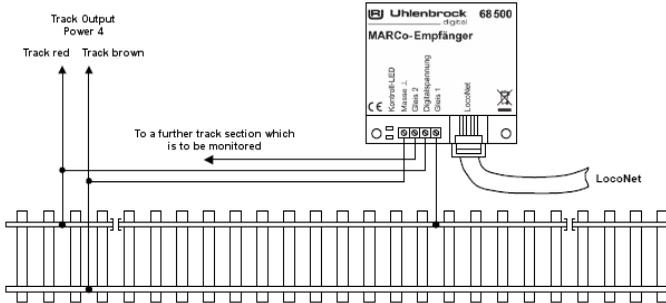
For simple train monitoring in two places with a module the following functions must be programmed:
