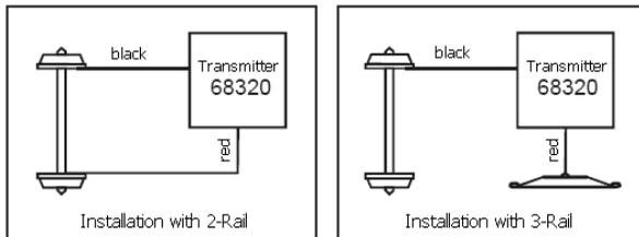
Connect the wires of the MARCO transmitter to the power pickup of your locomotive: the red wire with the right (isolated) pickup of its locomotive, the black wire with the left (non-isolated) pickup.
