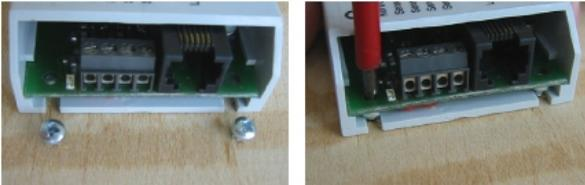
Fasten the MARCo-Receiver in the proximity of the detectors under your layout. Position the MARCo-Receiver under the layout board and mark the mounting holes of the module. Turn two screws (round head screws  $\varnothing 2.5 \times 10$ ) so far into the board that they will still push into the slots of the MARCo-Receiver.
